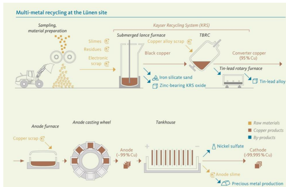
Figure 5 - Treatment process at Aurubis (Lünen, Germany)
